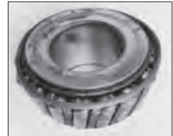
Cone large rib face deformation Metal flow from excessive heat generation.
