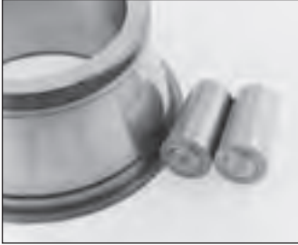
Abrasive wear Fine abrasive particle contamination.
