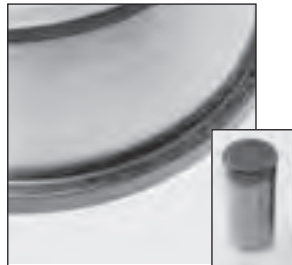
Cone large rib face scoring Welding and heat damage from metal-to-metal contact.
