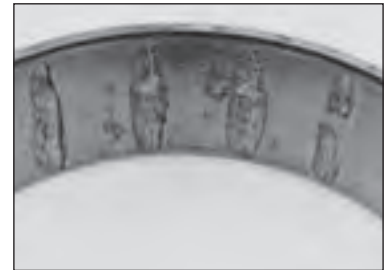
Line spalling Roller-spaced spalling from bearings operating after etching damage.
