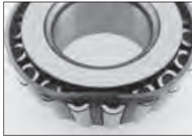
Cage deformation Improperly installed or dropped bearing.
