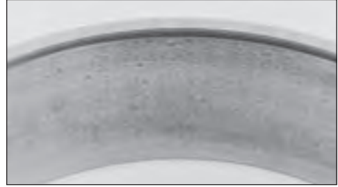
Bruising Debris from other fatigued parts, inadequate sealing or poor maintenance.
