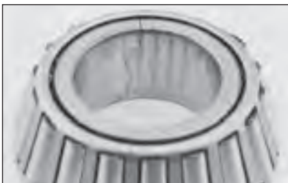
Cone bore damage Fractured cone due to out-of-round or oversized shaft .
