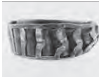
Total bearing lock-up Rollers skew, slide sideways and lock-up bearing.
