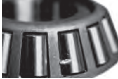
Grooving Large particle contamination imbedding into soft cage material.
